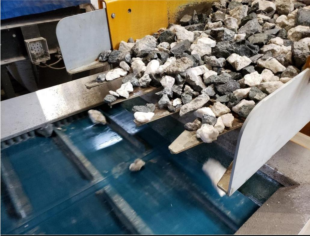
Figure 2. Steinert KSS sorter with XRT colour laser induction
